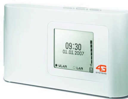
Figure 4:UMTS-router that provides access to several devices (XSB0x R4v)
